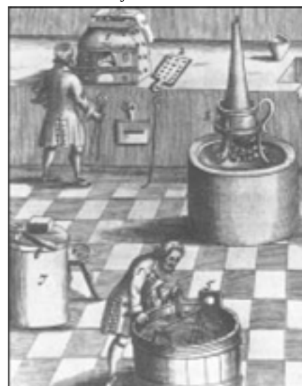
Figure 7 - Density measurement (foreground) in London, 17th century. Fire assay can be seen behind (from reference 1)
